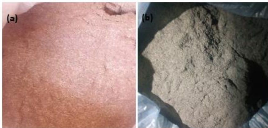
Figure 1. Images of (a) Milled coconut shells; (b) Carbonized coconut shell particles.
