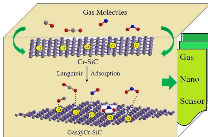
Figure 1. A simulated box of Langmuir adsorption of CO, CO 2 , NO, and NO 2 onto Cr-doped SiC nanosheet towards the formation of gas adsorption.
