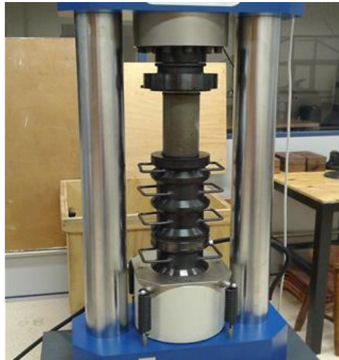
Figure 3. Compressive strength test in progress.
