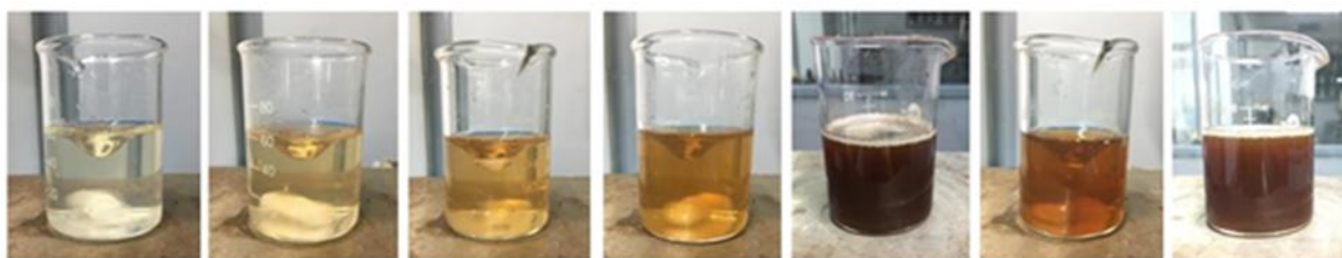
Figure 1. Synthesis of Sesbania Sesban silver nanoparticles – color change in the reaction mixture.
