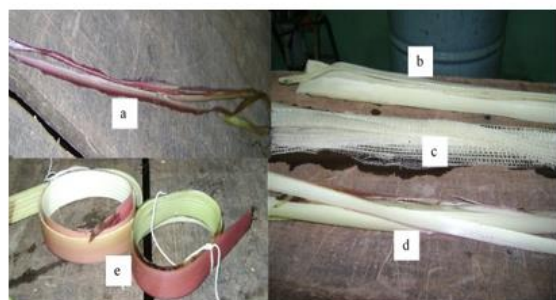
Figure 2. A sequence of obtaining and separation of the different types of fibers in the banana tree log: (a) “Limit part fiber” ( F_{lim} ), (b) “External lateral part fiber” ( F_{Lext} ), (c) “Internal part fiber” ( F_{int} ), (d) “Intermediary part fiber” ( F_{interm} ) and (e) “External part fiber” ( F_{ext} ).
