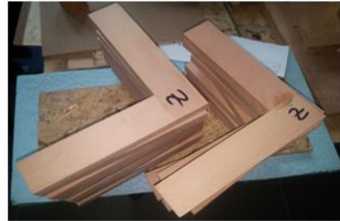
Figure 4. Prepared corner-joint specimens.
