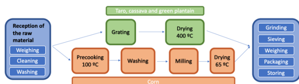
Figure 1. Scheme of the sample preparation.
