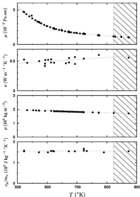
Figure 4. Thermophysical properties of eutectic NaNO3 / KNO3. ( by the authors).
