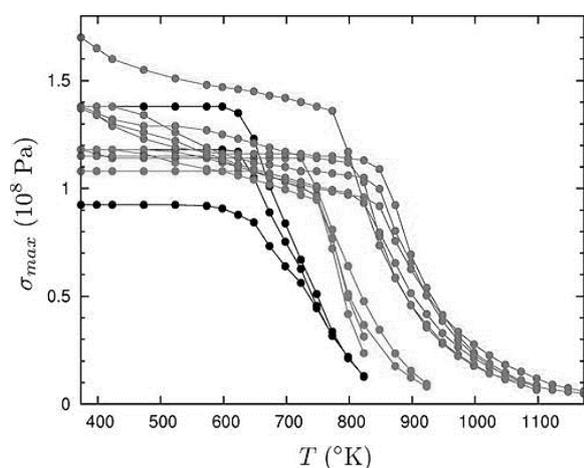
**Figure 2.** Maximum steel stress permitted by boiler and pressure vessel adapted from ASTM E2860-12 ( by the authors).
